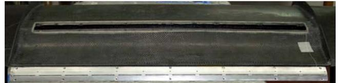
**Figure 2: A rear-view of the airplane wing, the opening for the actuators and the actuators' exit slots before being installed in the wing. Twelve actuators were installed in each wing.**
