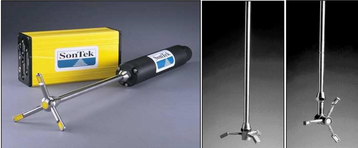
Figure 2. Acoustic Doppler Velocimeter (ADV) and 3D probes.
