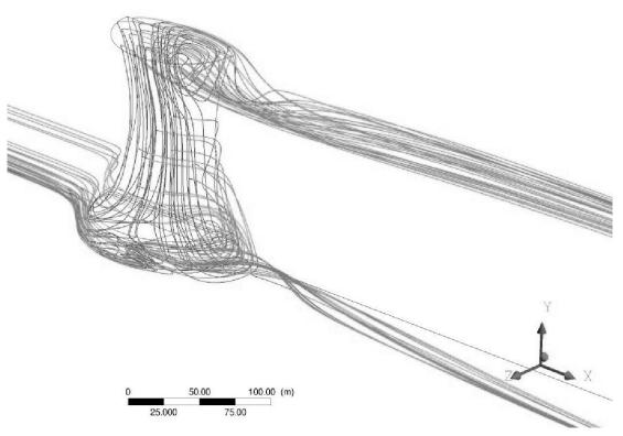
Fig. 2. Streamlines in the case of crosswind configuration
