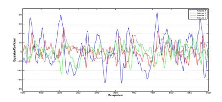
Obrázek 2: Example of temporal evolution of expansion coefficients for four POD modes. Each colour corresponds to one POD mode.
