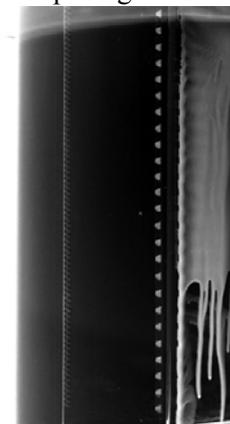
**Figure 5** triangular VGs ( $h_2, x_2, \Delta z_1$ ), zig-zag tape,  $\gamma = 20$  deg.
