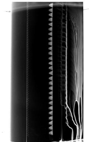
**Figure 4a** rectangular VGs ( $h_2, x_1, \Delta z_2$ ), zig-zag tape,  $\gamma = 20$  deg.
