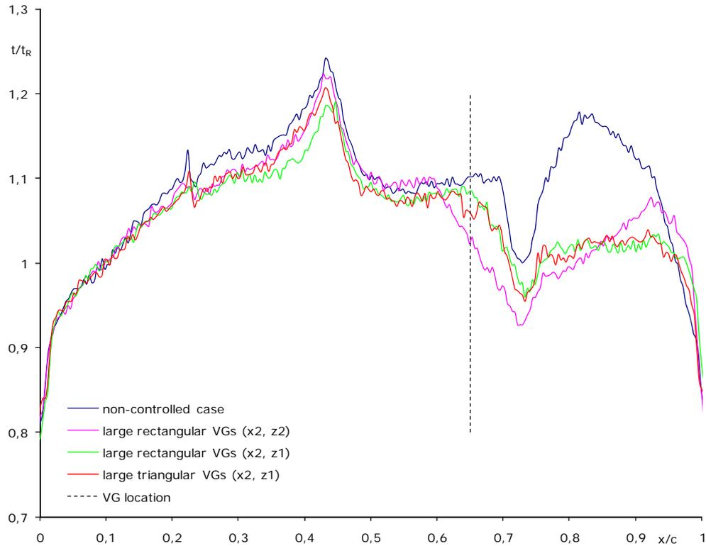
Figure 8 Comparison of non-dimensional temperature distribution over airfoil surface with zig-zag tape,  $\gamma = 20$  deg.,  $\alpha = 0$  deg.
