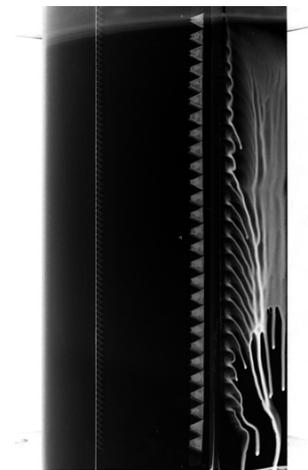
**Figure 4b** rectangular VGs ( $h_2, x_2, \Delta z_2$ ), zig-zag tape,  $\gamma = 20$  deg.
