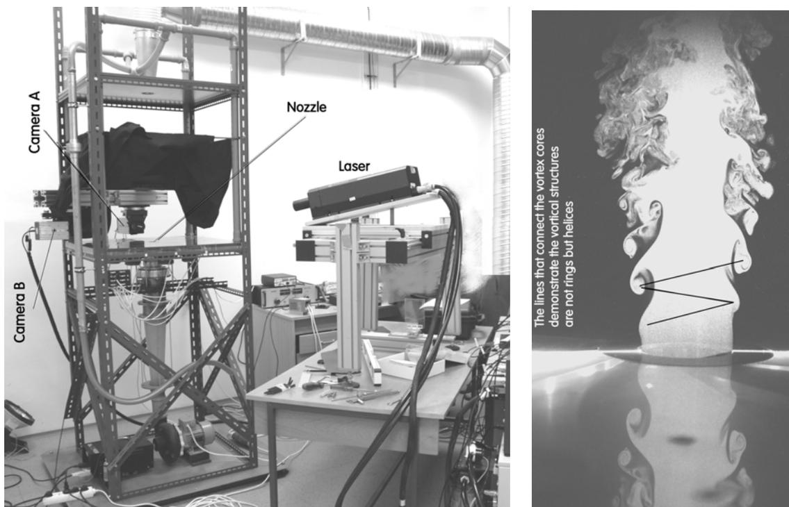
Fig. 1 (Left): The experimental setup for the PIV data acquisition. The black curtains surrounding the jet are here lifted to reveal the nozzle exit. **Fig. 2 (Right)**: A typical example of the investigated jet:  $Re = 8.0 \cdot 10^3$ , excitation frequency 62.8 Hz (Both photographs: P. Antoš)
