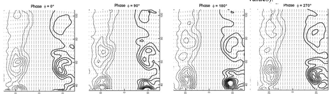
Fig. 4 (Below) Another example of a sequence: phase-averaged distributions of vorticity (dashed lines at left-hand sides of images represent negative values).
