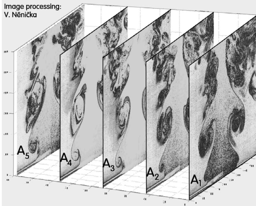
Fig. 3 (Left) Image acquisition synchronised with the excitation makes possible study of the progressive phases of the structure development. In this example of a sequence at increasing phase angle, it may be interesting to follow the vertical motion and growth of the section through the vortex from  $A_1$  to  $A_5$ .
