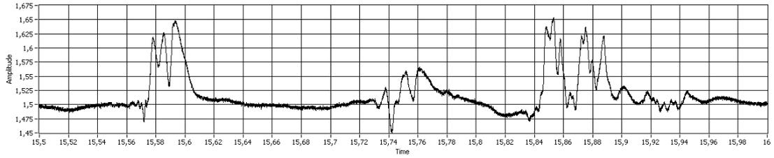
Fig. 1 Raw voltage signal from CTA in duration 0,5s
