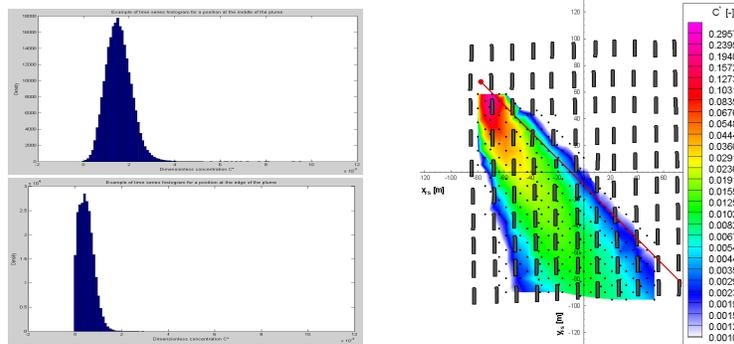
Figure 2: Examples of dimensionless concentration histograms (plume centre upper left, plume edge lower left) and mean concentration distribution at half building height within the MUST set-up.
