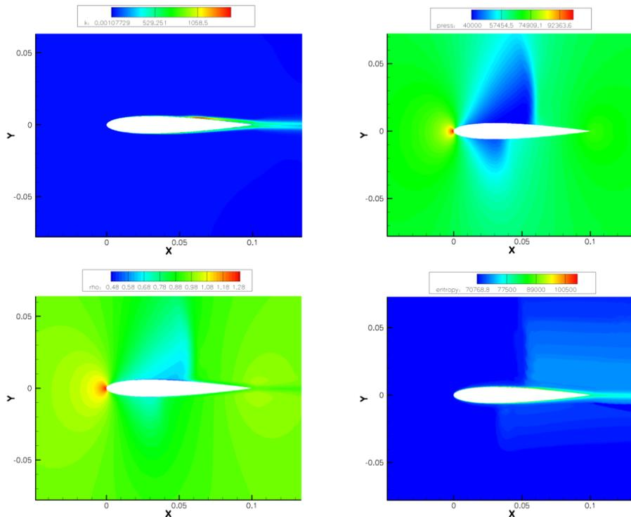
Figure 2: Nonstationary turbulent flow,  $k$ , pressure, density and entropy isolines, solution after 18.900.000 iterations
