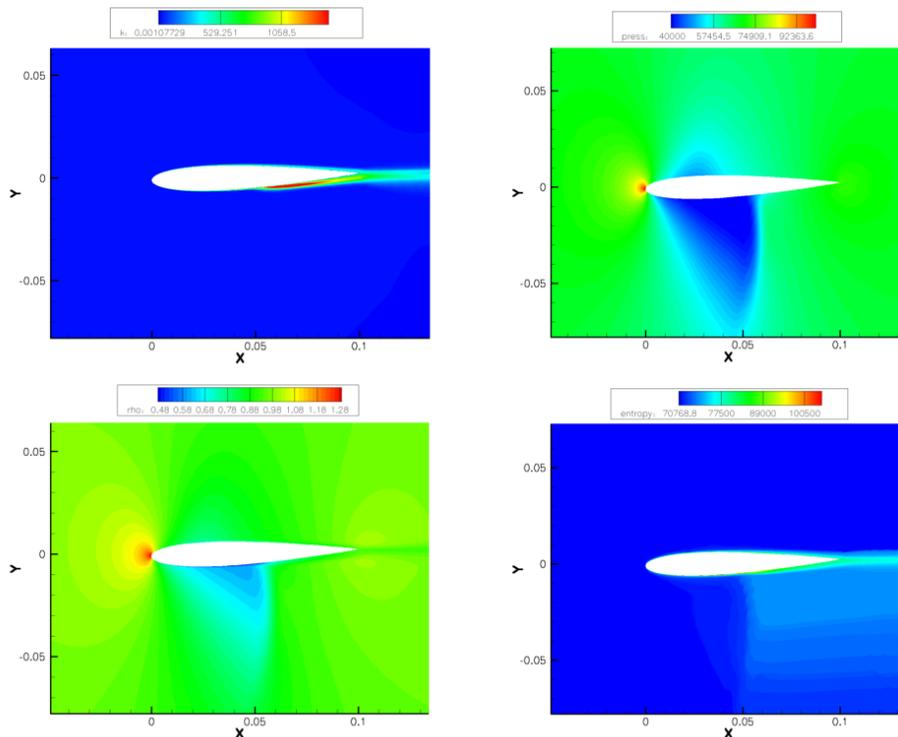
Figure 4: Nonstationary turbulent flow,  $k$ , pressure, density and entropy isolines, solution after 78.000.000 iterations
