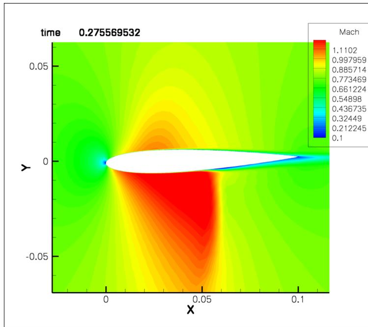
Figure 3: Nonstationary turbulent flow, Mach number isolines, solution after 78.000.000 iterations
