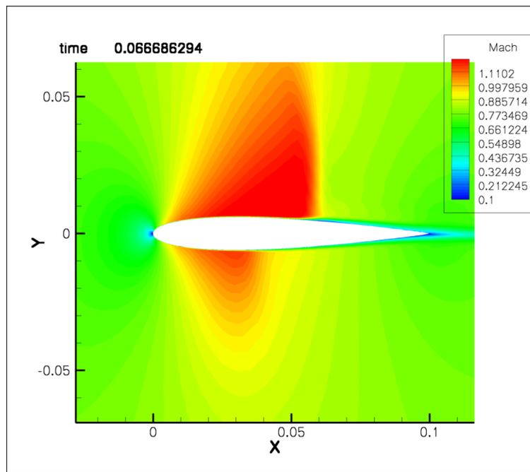
Figure 1: Nonstationary turbulent flow, Mach number isolines, solution after 18.900.000 iterations
