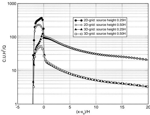
Fig 1: Ground-level-concentrations with source at heights  $0.25H$  and  $0.5H$  showing the effect of terrain amplification factor and pollutant plume decay in 2D-case (upper two profiles) versus 3D-case on domain-1 (lower two profiles).
