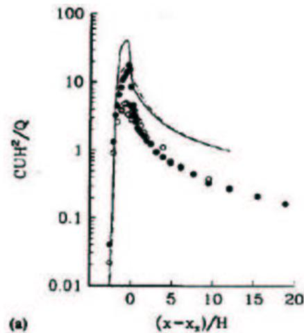
Fig 2: Castro's reference data (solid line) based on 3D-calculation from [2] pp.847: Profile of ground-level-concentrations profiles with source at heights  $0.25H$  and  $0.5H$ , normalized as  $C \cdot U_0 H^2 / Q$ .
