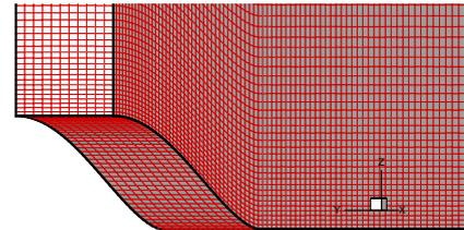
Fig 8: Zoom to 3D-computational domain-1 for 3D-concentration field discretized by  $200 \times 11 \times 80$  cells.
