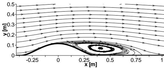
Fig 5: Zoom to separation zone behind hill, computed reattachment  $x_r = 6.84H$ , measured from experiment  $x_r = 6.5H$ .
