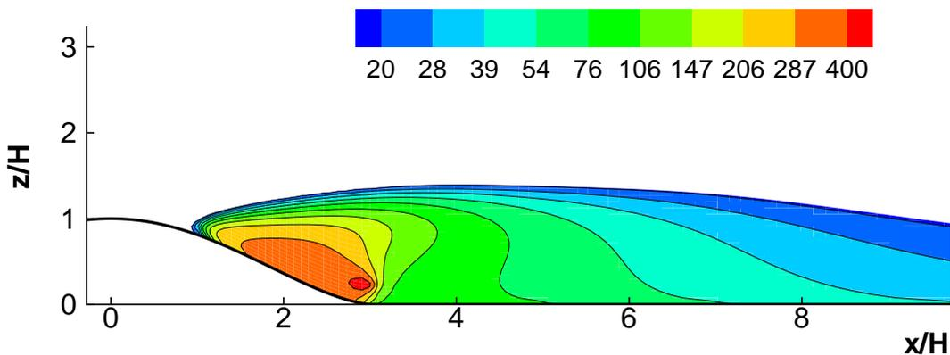
Fig 9: Computed contours of normalized 2D-concentration field  $C \cdot U_0 H^2 / Q$  with exponential scale for source height  $0.25H$ .
