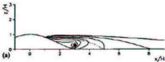
Fig 11: Reference data taken from [2] pp.847: Computed contours of normalized concentration field  $C \cdot U_0 H^2 / Q$  with exponential scale starting at value=1 (upper contour) for source height  $0.25H$ .
