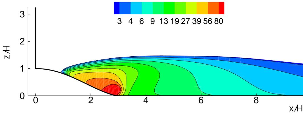
Fig 10: Computed contours of normalized 3D-concentration field  $C \cdot U_0 H^2 / Q$  with exponential scale for source height  $0.25H$ , middle XZ-plane at index  $J=6$ .
