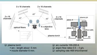
DISTRIBUTIONS OF PLASMA RADIATION: MEASURED IN PLANE A - OUTSIDE AND PLANE B - INSIDE THE TORCH (THROUGH SILICA WALL).
