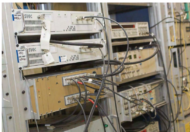
Fig. 1. A SAW-filter-excitation time-interval meter developed at ÚRE has been used for the first time in the GPS GTR50 timing receivers also developed at ÚRE (the two light-colored instruments on the upper left-hand side).
