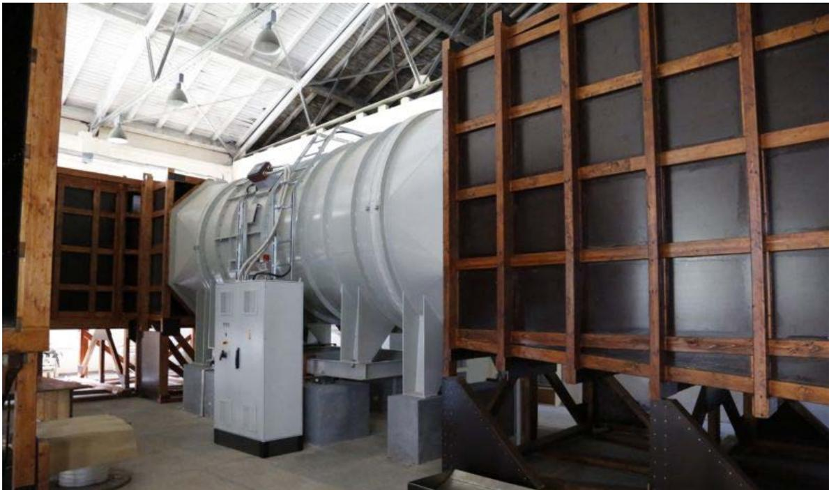
Fig . 2 Overview of the WT power unit and its control system.
