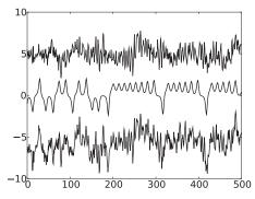
FIG. 1. A sample of the analyzed time series. The curves from top to bottom: the AR(5) process, the *x*-coordinate of the Lorenz oscillator, and the mixed signal. The Lorenz signal is not introducing any clear oscillatory activity into the linear autoregressive process at the given time scale. Signals have been shifted for clarity.
