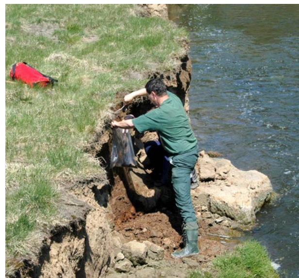
■ Fig. 42. Sampling of contaminated floodplain sediments of the Litavka River below the Příbram Ore Region. Photo by J. Brožek.
