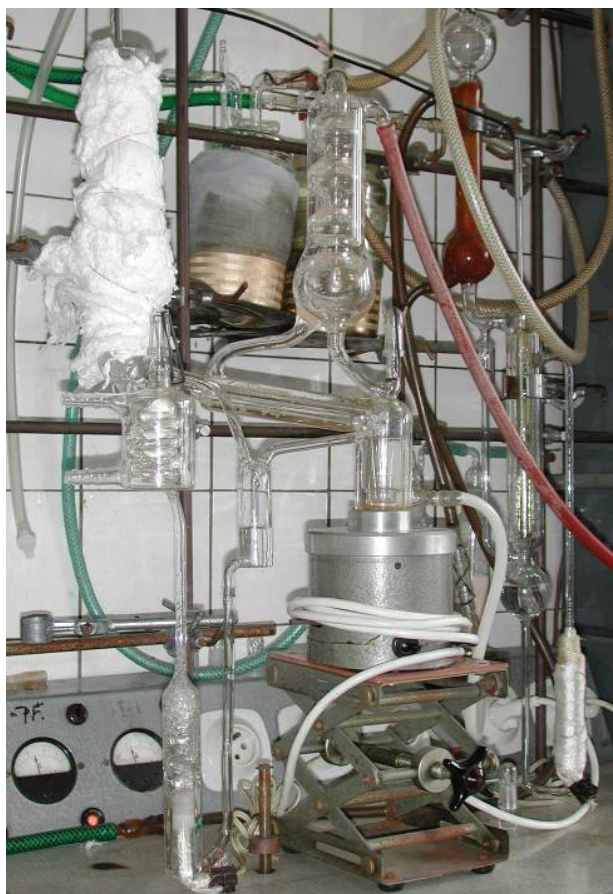
All glass recirculation still for VLE measurement
