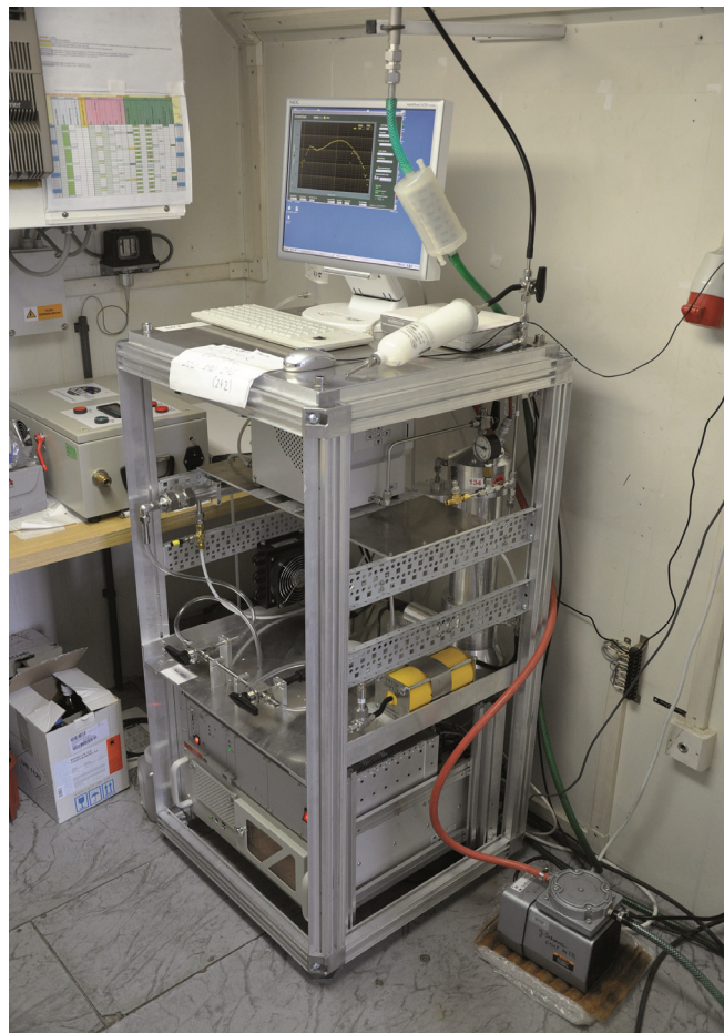
A photo of scanning mobility particle sizer measuring size distribution of particles at background site Košetice
