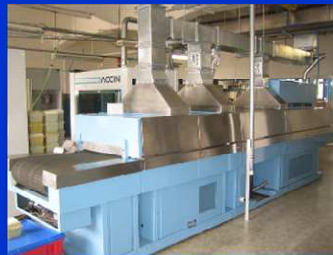
Infrared belt furnace (6 independent zones)
