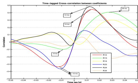
Obrázek 3: Time-lagged cross-correlation between particular expansion coefficients (e.g. R12=correlation between expansion coefficients of Mode 1 and Mode 2). Thick line labels the correlations with significant maximum.
