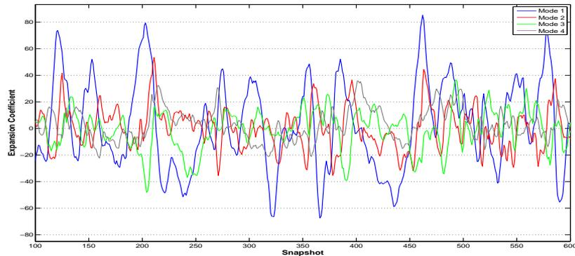
Obrázek 2: Example of temporal evolution of expansion coefficients for four POD modes. Each colour corresponds to one POD mode.
