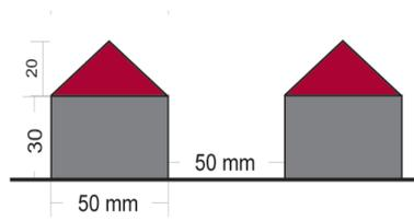
Obrázek 1: Side-view of the street canyon inside the wind-channel.
