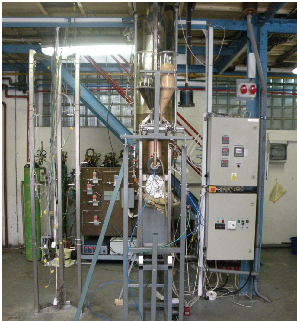
Fluidized bed gasifier
