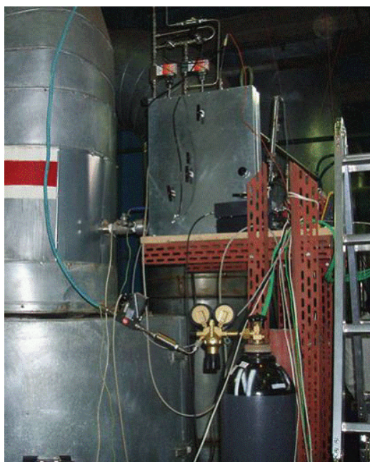
Aerosol sampling train connected to the turbine at thermal power plant Pruněřov II
