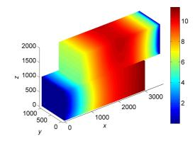
Figure 2: Distribution of von Mises stress.
