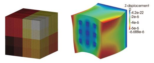
Figure 1: Example of a division of the cube into 64 subdomains (left) and (magnified) deformed shape for contrast  $E_2/E_1 = 10^6$  coloured by vertical displacement (right). Reproduced from [8].
