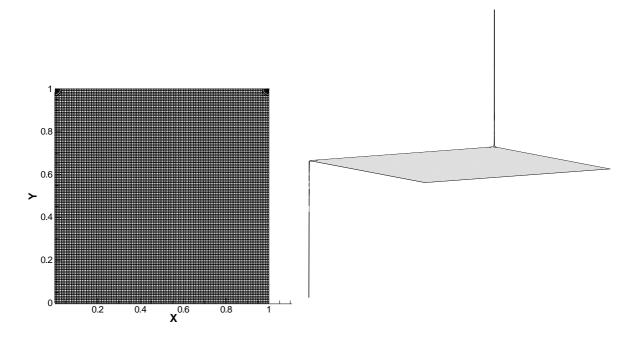
Figure 3: Lid driven cavity, Re = 10,000 Left: mesh 128×128 refined locally Right: pressure.
