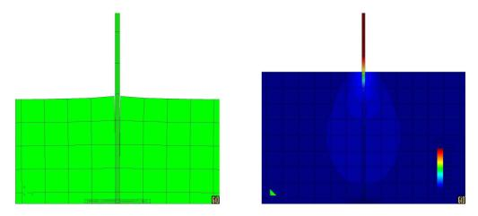
Figure 1: Detail of deformed shape and stress distribution.
