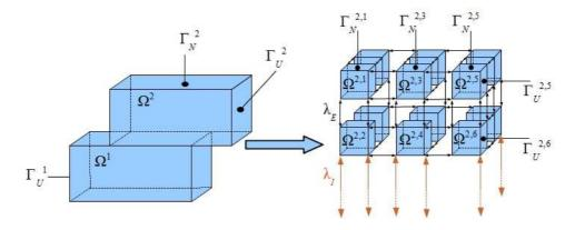
Figure 1: Scheme of the geometry and domain decomposition.
