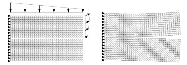
Figure 1: Contact of two elastic bodies  $\Omega^1$  (the upper body) and  $\Omega^2$ , along the contact boundary  $\Gamma_c$ . The loading is due to the surface traction. On the right: Resulting displacements.
