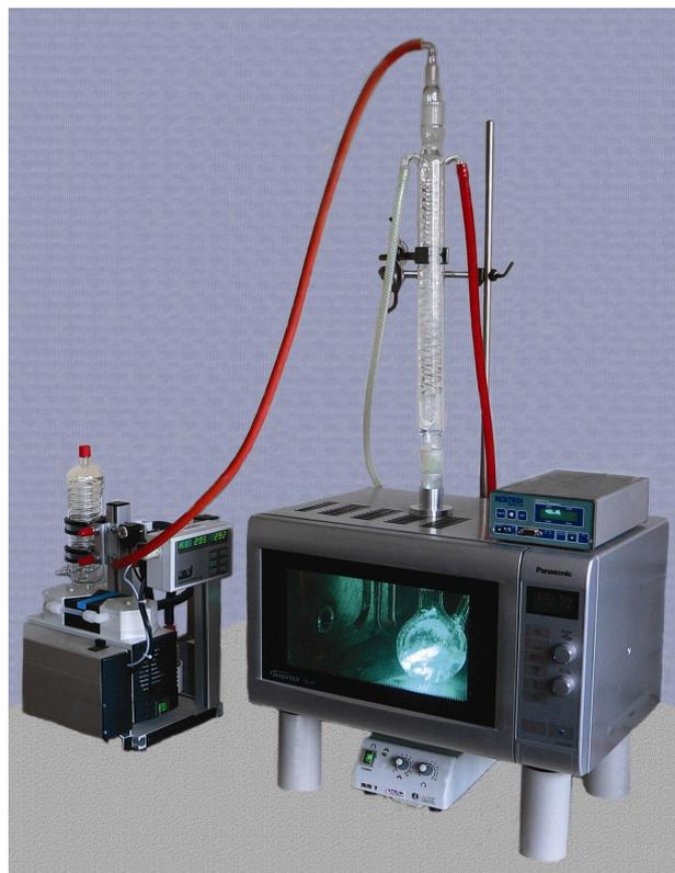
Figure 1. Low-pressure batch microwave photoreactor.
