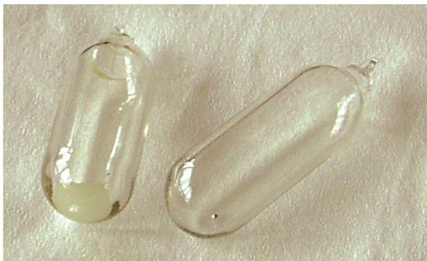
Figure 3. Hg-EDL and S-EDL for photochemical applications.
