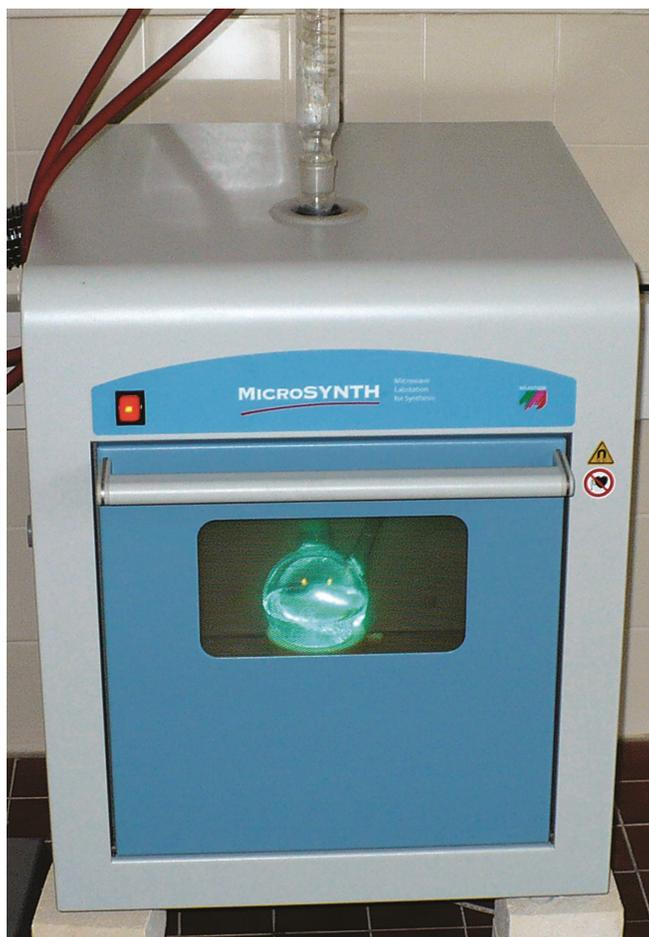
Figure 16. Microwave photocatalysis arrangement on Milestone's MicroSYNTH Labstation.
