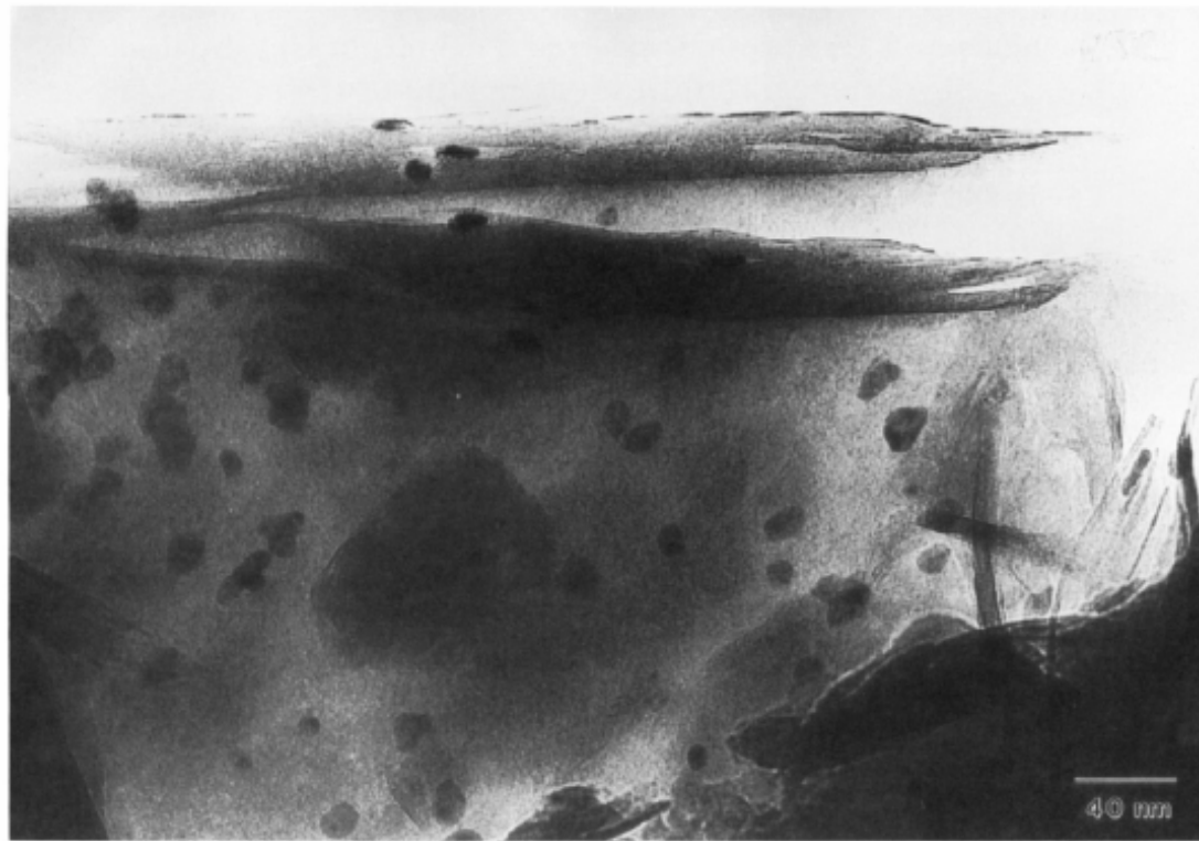
Figure 1. Transmission electron micrograph of 1. Folding of the clay layers (through ca. 90°) at the clay particle edge is apparent.
