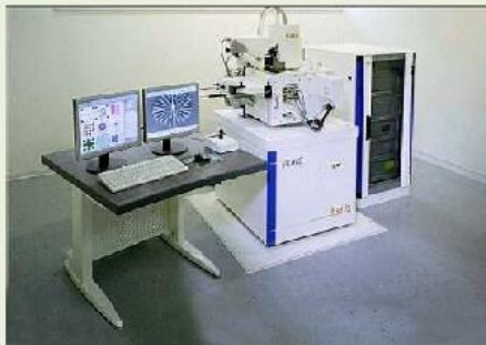
EBL using "e-LiNE system" (Raith GmbH)
