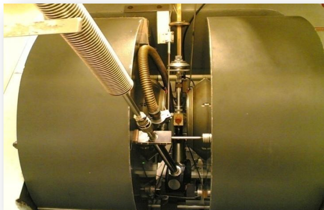
Fig. 2. Magnet system and resonant cavity between the poles magnet
