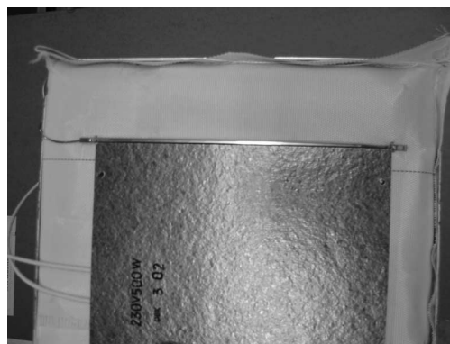
Placement of the capillary tube sensor on the heating element
