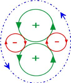
Figure 4. Cross section through the first developmental stage of a dissipative patch, i.e. of an unstable pair of likewise rotating vortices resulting from a dipole-dipole collision (right pathway in figure 1). The green circles represent primary energy-containing vortices. They do not touch each other due to spontaneously formed secondary vortices which initiate a whole vortex cascade. The broken blue line and the arrows symbolize the slow rotation of the patch around its center of mass.
