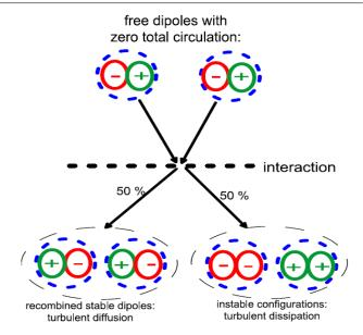
**Figure 1.** Collisions of two dipoles: the left pathway is 'diffusive'; it is a recombination of dipole elements and chaotically scatters the trajectories (turbulent diffusion). The right pathway is 'dissipative'; it evolves into an unstable vortex configuration which decays 'somehow' into heat.
