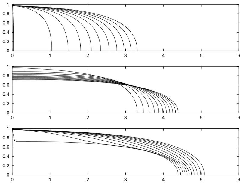
Figure 1. Effective saturation ( $u$ ) profiles vs. distance  $x$  in cm, for the sand soil under consideration, every 18 minutes, for (topmost) the initial horizontal wetting, (middle) centrifugation with insulated end, (bottom) the final horizontal wetting.
