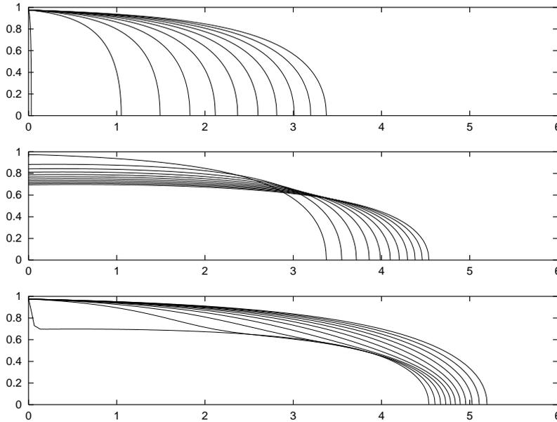
Figure 6. Effective saturation ( $u$ ) profiles vs. distance  $x$  in cm, for the sand soil under consideration, every 18 minutes, for (topmost) the initial horizontal wetting, (middle) centrifugation with an insulated end, (bottom) the final horizontal wetting.
