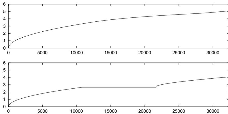
Figure 2. The corresponding evolution of (top) the interface position  $s$  in cm, (bottom) the total flux input  $Q$ , vs. time in seconds.
