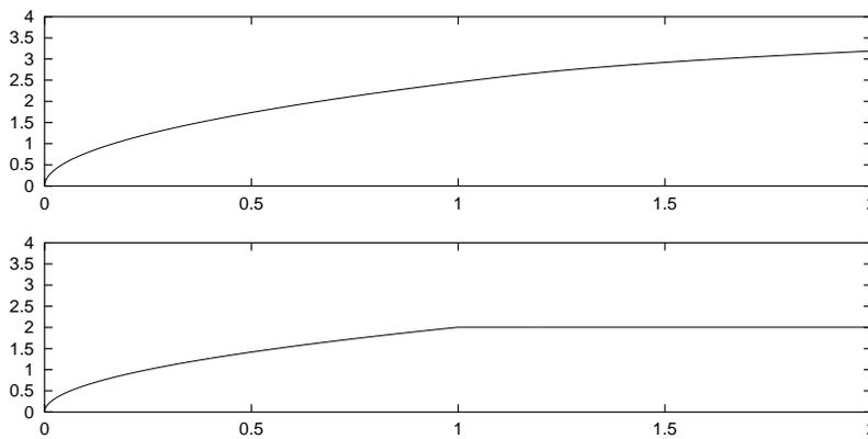
Figure 5. The corresponding evolution of (top) the interface position  $s$ , (bottom) the total flux input  $Q$ , vs. time.
