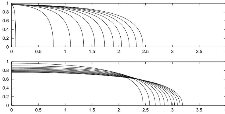
Figure 4. Effective saturation ( $u$ ) profiles vs. distance  $x$ , for the example parameters under consideration, every 0.1 time units, for (topmost) the initial horizontal wetting, (bottom) gravitation.
