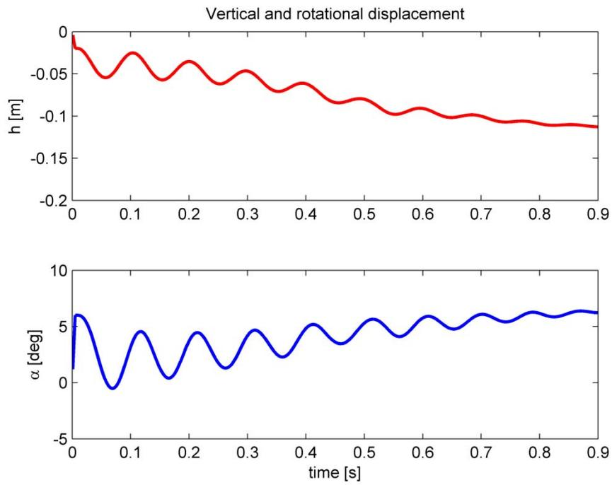
Figure 7: Vertical displacement and angle of rotation in dependence of time for  $U_\infty = 35 \text{ m.s}^{-1}$
