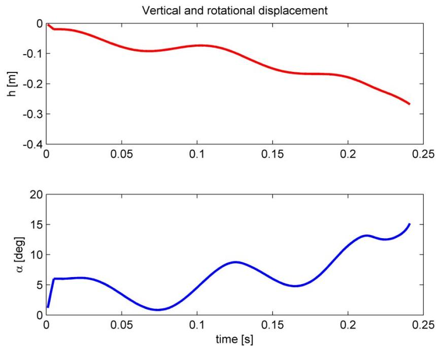
Figure 8: Vertical displacement and angle of rotation in dependence of time for  $U_\infty = 40 \text{ m.s}^{-1}$
