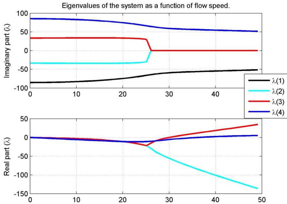
Figure 4: Real (up) and imaginary part (bottom) of eigenvalues of the system as a function of a flow speed.
