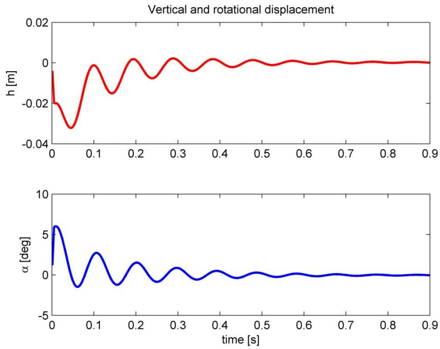
Figure 6: Vertical displacement and angle of rotation in dependence of time for  $U_\infty = 29 \text{ m.s}^{-1}$
