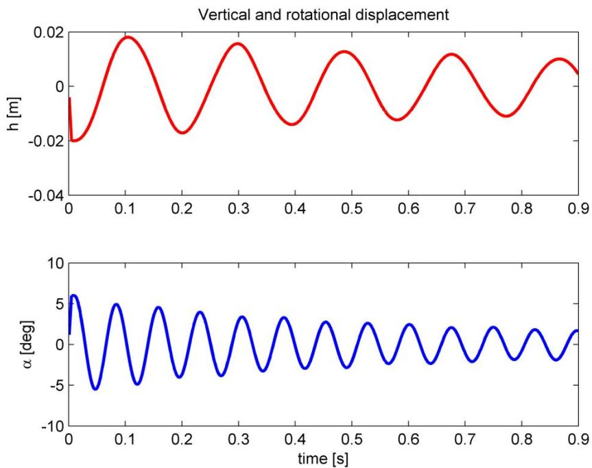
Figure 5: Vertical displacement and angle of rotation in dependence of time for  $U_\infty=0 \text{ m}\cdot\text{s}^{-1}$
