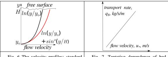
Fig. 6 The velocity profiles: standard averaged turbulent profile (the log-law) and profile with influence of the flow depth and wavy surface. Fig. 7. Tentative dependence of bed load transport rate,  $q_s$ , on flow velocity,  $u_*$ .
