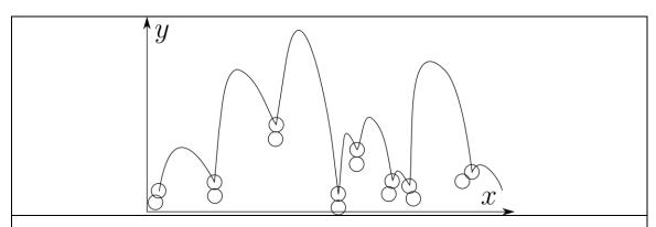
Fig. 5 A hypothetical trajectory of the saltating particle after its collisions with other conveyed particles and bed particles.
