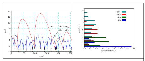
Fig. 1 Saltation of one particle with various flow velocities: effect of shear velocity on trajectory. Fig. 2 Normalized concentration of the saltating particles in the separate layers [0-2; 2-4; ...] d for various flow velocities,  $u_*$ . Depth of the flow is H = 20 d.
