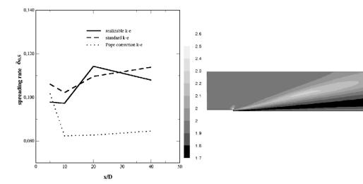
In the Figure 1 non-reacting flow calculations of jet spreading rates are presented. Figure 2 shows local changes of the  $C_{\epsilon 2Pope}$  coefficient calculated in the flow filed area of the jet.
