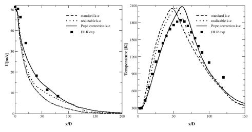
Fugure 3. Axial velocity and temperature in the centerline.
