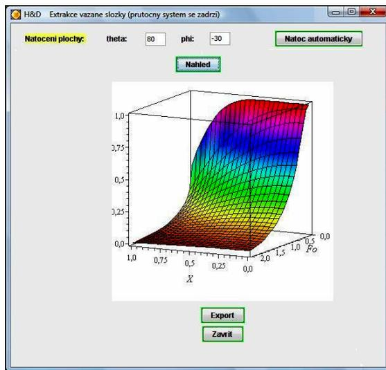
FIG. 2 Window for view and export of dimensionless concentration field in solid phase like a function of position and time
