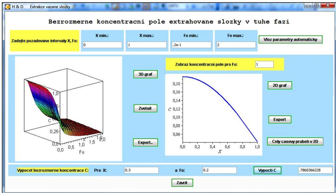
FIG. 1 Window for solving and visualization of dimensionless concentration field in solid phase
