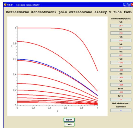
FIG. 3 Window for view and export of dimensionless concentration field in solid phase like a function of time
