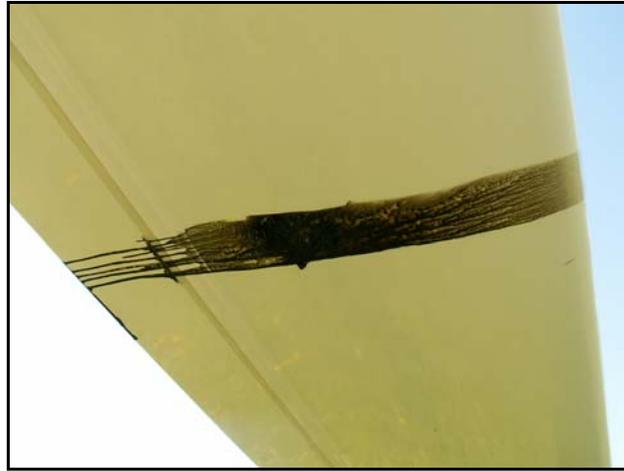
Fig. 4 Oil-flow visualization on lower surface of outer wing segment of TST10a sailplane, in the aileron region.  $V = 100\text{ km/h IAS}$ . Right to left: laminar boundary layer, separation bubble, turbulent boundary layer
