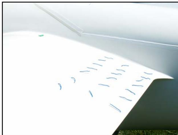
*Fig. 3 Array of tufts and vortex generator installed on the left wing root of TST10a prior to the test flight*
