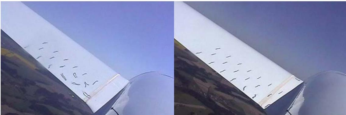
Fig. 5 Tuft visualization on left wing root of TST10a,  $V = 85\text{ km/h IAS}$ . Left figure – uncontrolled case, note large region of separated flow. Right figure – VG1 applied, attached flow till the proximity of wing trailing edge
