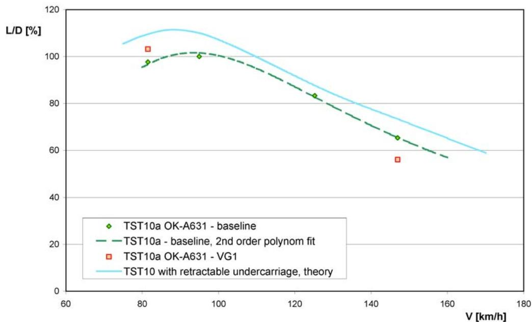
Fig. 6 Measured L/D performance of TST10a sailplane – baseline, VG installed and theoretical prediction. Wing loading,  $m/S = 31.4 \text{ kg/m}^2$
