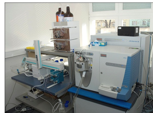
LTQ Orbitrap XL (Thermo) Small molecules, biomolecules (HR); ESI, APCI, nanoESI
