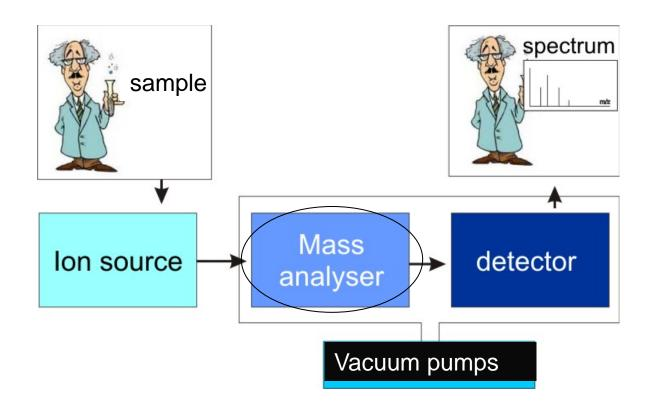
• Mass analysers - separate the ions according to their mass-to-charge ratio
