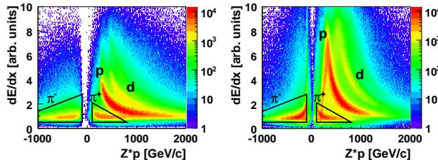
**Fig. 1:** Distribution of the energy loss versus charge\*momentum of particles detected in inner TOFINO (left) and outer TOF (right) detectors
