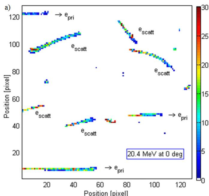
**Figure 1.** Detection of individual relativistic electrons with energy 20.4 MeV at 0 by Timepix in TOT mode. The beam was incident from left. The energy measured per pixel is given by the vertical bar shown in color in keV. Data frames collected in 10 ms. Only a quarter (128×128 pixels) of the full sensor area is shown.
