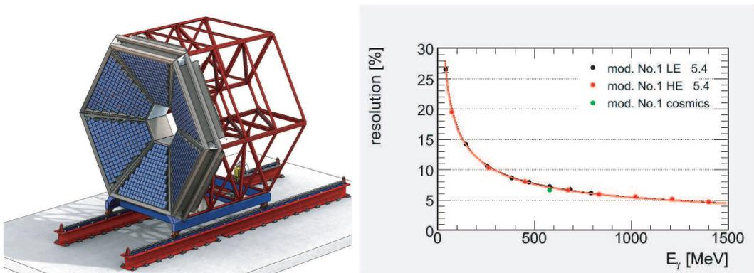
**Fig. 1: Left: 3D view of the Calorimeter model. Right: Energy resolution of lead glass measured with photon beams as a function of photon energy.**
