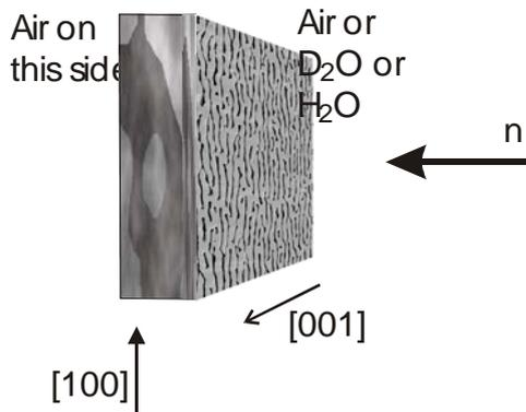
Fig. 1. Membrane and its orientation for double-crystal SANS experiment.
