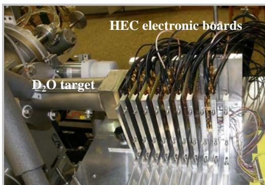
*Neutron hardness test experiments of HEC read-out electronics\** are currently provided using the high-power  $p\text{-D}_2\text{O}$  neutron source. The program is supported by the NRD/MPI München Contract (2008-12) within the ATLAS Collaboration. To perform the radiation tests of HEC read-out
