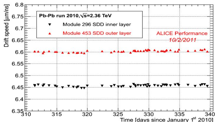
Figure 1: Drift speed in two selected SDD modules as a function of time during Pb-Pb 2010 data taking. The difference of average values between inner and outer layer is due to different temperature on the two layers.
