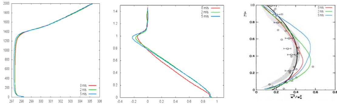
Fig 1. Vertical profiles for CBL a) final temperature profile b) heat flux scaled by it's surface value c) vertical velocity variance scaled by  $w_*$ . In b) and c) height is scaled by  $z_i$  (adapted from Holtslag and Moeng, 1991)
