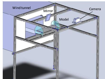
Fig. 1. Schema of the experimental setup for oil flow visualization.
