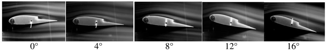
**Fig. 13. Smoke visualization results for the 2415-6 airfoil from 0 to 16 deg. of AOA.**
