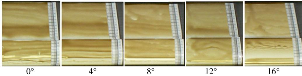
Fig. 6. Oil visualization results for the 2415-4 airfoil from 0 to 16 deg. of AOA.
