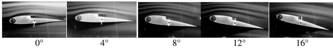
**Fig. 11. Smoke visualization results for the 2415-4 airfoil from 0 to 16 deg. of AOA.**
