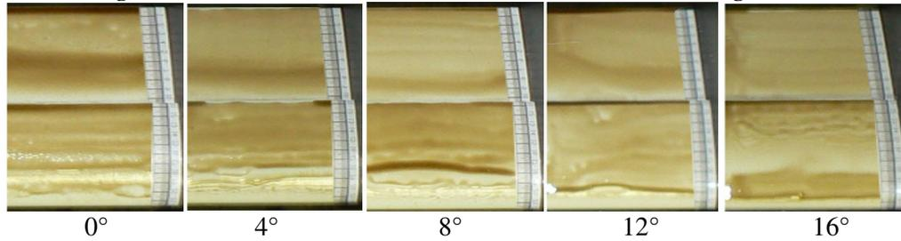
Fig. 7. Oil visualization results for the 2415-5 airfoil from 0 to 16 deg. of AOA.
