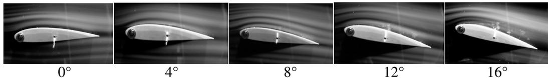
**Fig. 14. Smoke visualization results for the NACA 2415 airfoil from 0 to 16 deg. of AOA.**
