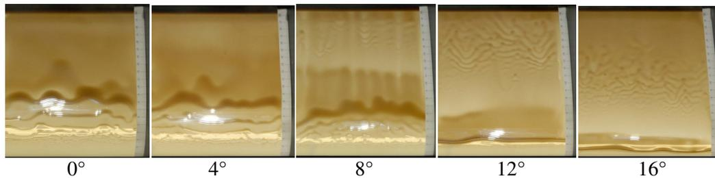
Fig. 9. Oil visualization results for the NACA 2415 airfoil from 0 to 16 deg. of AOA.
