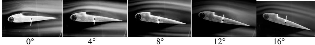
**Fig. 10. Smoke visualization results for the 2415-3 airfoil from 0 to 16 deg. of AOA.**
