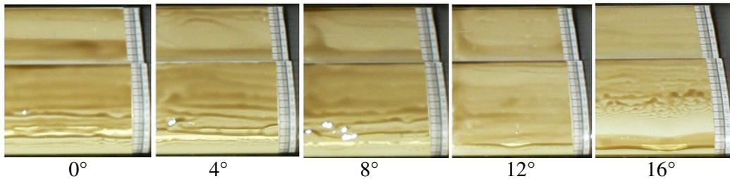
Fig. 8. Oil visualization results for the 2415-6 airfoil from 0 to 16 deg. of AOA.
