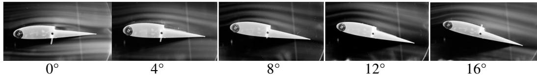
**Fig. 12. Smoke visualization results for the 2415-5 airfoil from 0 to 16 deg. of AOA.**
