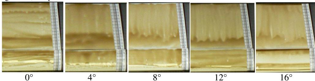
**Fig. 5. Oil visualization results for the 2415-3 airfoil from 0 to 16 deg. of AOA.**
