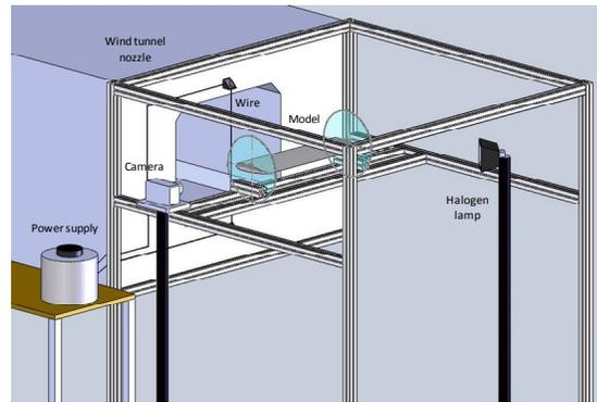
**Fig. 2. Schema of the experimental setup for smoke flow visualization.**
