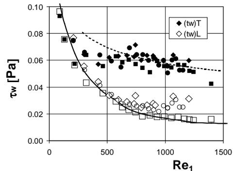
Figure 5. Conditional wall friction in smooth wall layers
