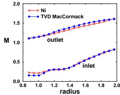
Fig. 6. Inlet and outlet Mach number distribution
