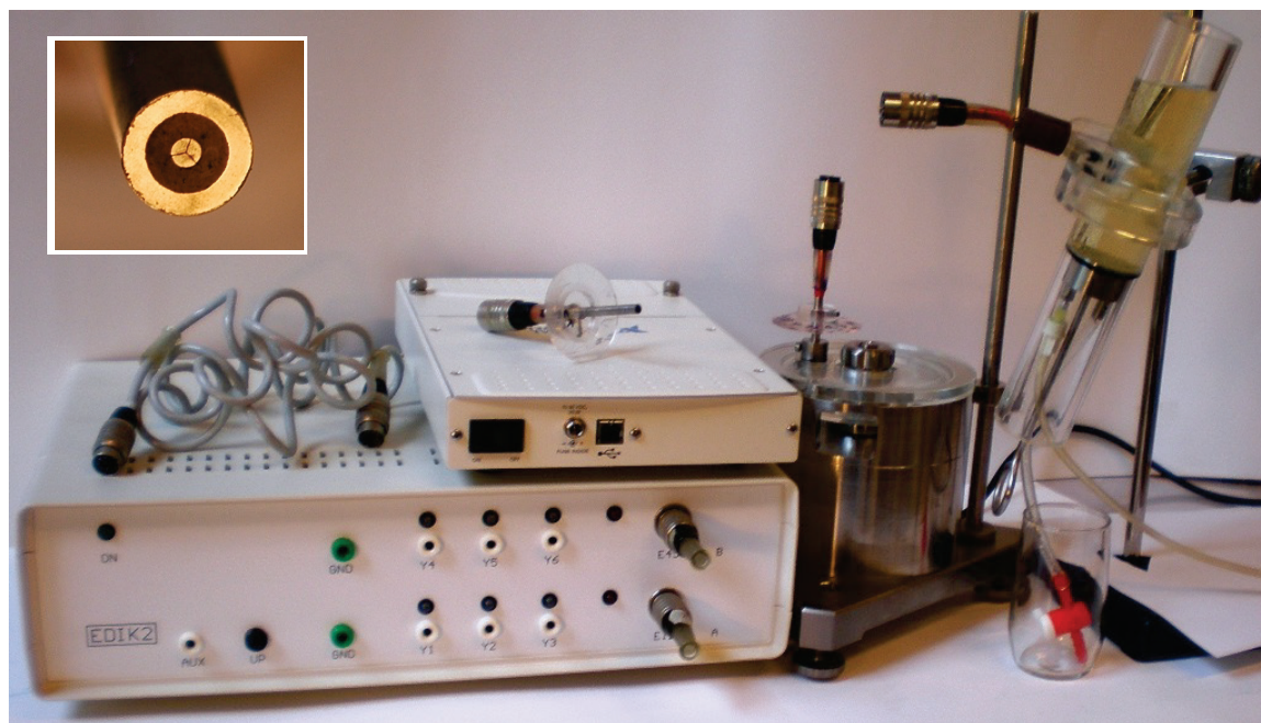
Setup for electrodiffusion experiments, used here in a voltamperometric study with three-segment electrodes
