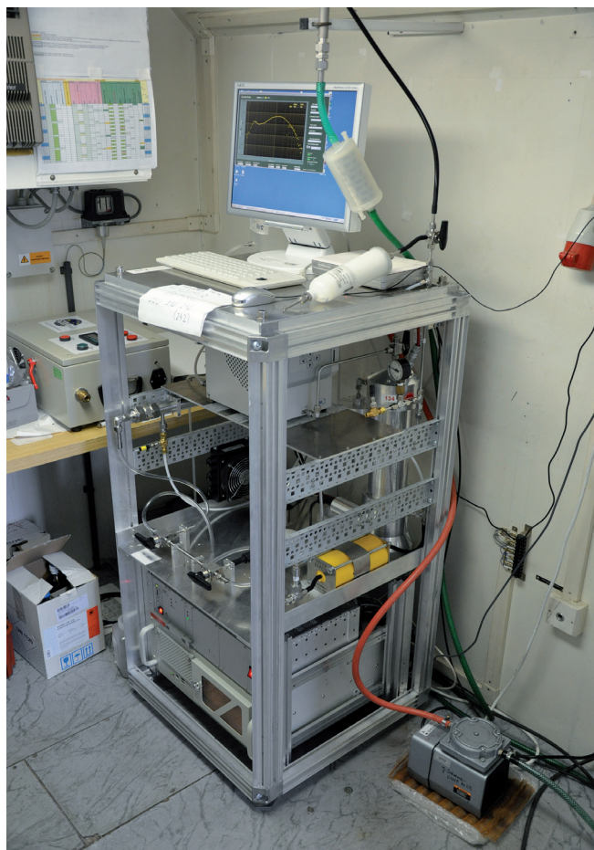
Photo of the scanning mobility particle sizer measuring size distribution of particles at background site Košetice
