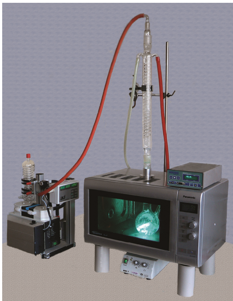
Experimental set-up for microwave photochemistry and photocatalysis
