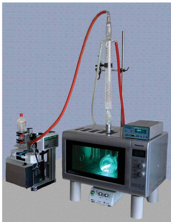
**Fig. (17).** Low-pressure batch microwave photoreactor [92].
