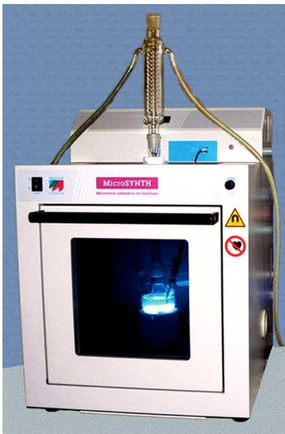
Fig. (4). Testing the EDL performance in a Milestone's MicroSYNTH Lab-station [32].
