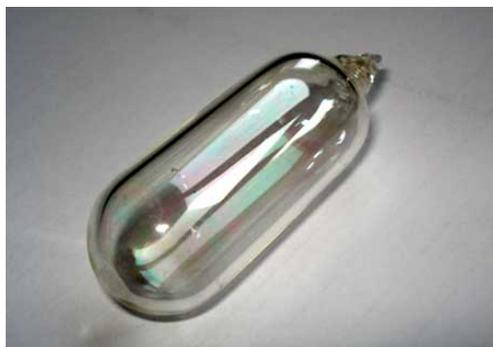
Fig. (6). Prepared titania-coated Hg-EDL.
