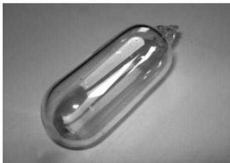
**Figure 14.6** Prepared titania-coated Hg-EDL.
