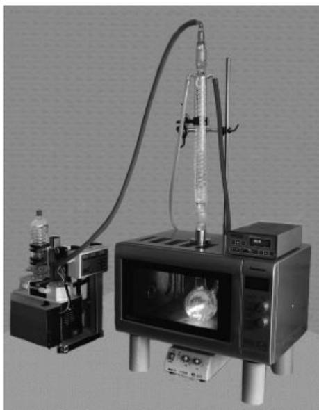
**Figure 14.19** Low-pressure batch MW photoreactor [105].
