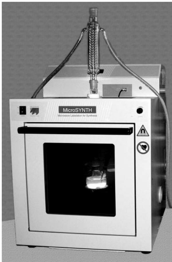
**Figure 14.4** Testing the EDL performance in a Milestone MicroSYNTH Labstation [30].
