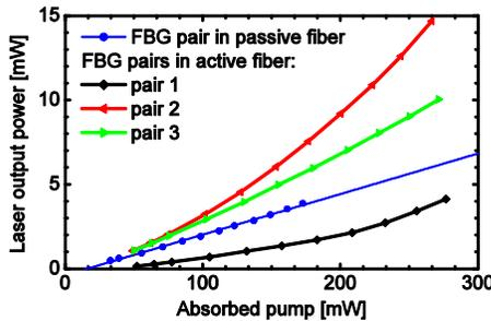
Fig. 3. Laser output vs. absorbed pump for the fiber laser with external FBG pair and for the monolithic configurations.
