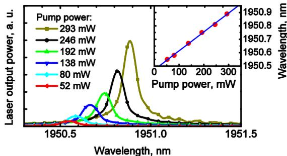
Fig. 4. Laser spectra of the monolithic TDFL with FBG pair No. 2 for various input pump power levels, Inset: Laser wavelength shift with the pump power together with linear fit.
