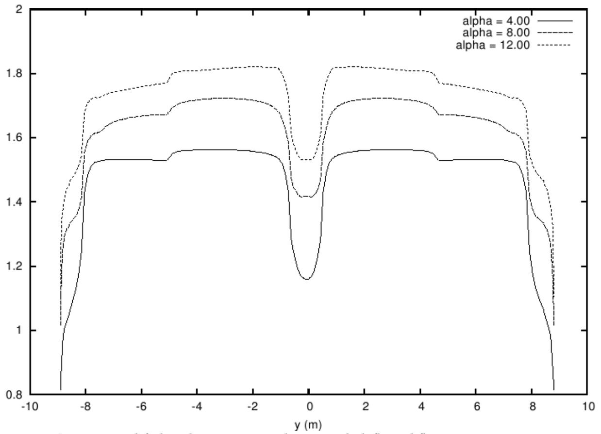
Illustration 5: spanwise lift distribution on a real wing with deflected flaps
