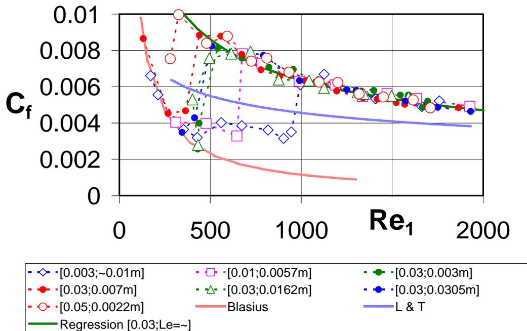
**Figure 2** Distributions of skin friction coefficient in boundary layers on rough surface (grids 80) under external turbulent flow
