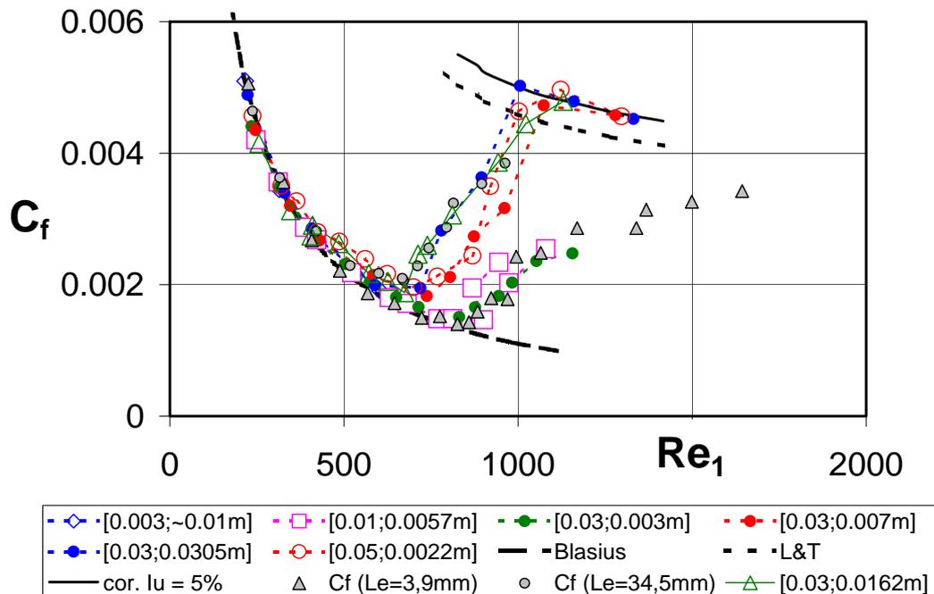
**Figure 1** Distributions of skin friction coefficient in boundary layers on smooth surface under external turbulent flow
