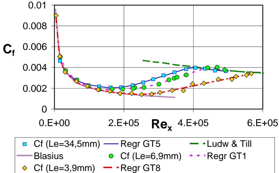
**Figure 4** Distributions of skin friction coefficient in boundary layers (grad  $P = 0$ ) under external grid turbulence flows with the intensity of velocity fluctuations  $I_{u_e} = 3\%$  at the onset of the layer  $x=0$
