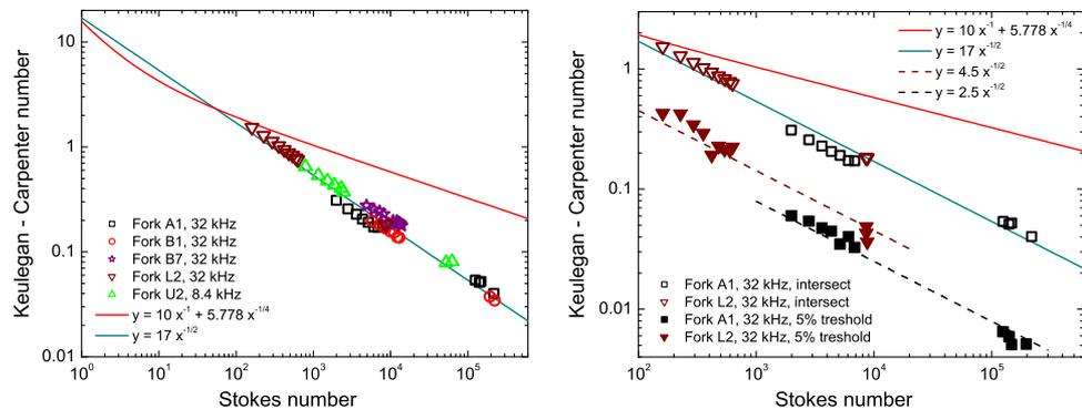
Obrázek 1: The cryogenic helium  $K_C$  versus  $\beta$  plots with  $K_C$  determined as a cross-section of limiting laminar and turbulent drag behaviour (left) and, for selected forks, using the criterion of 5 per cent deviation from linearity (right). The curved solid line represents expected instability for round cylinders.
