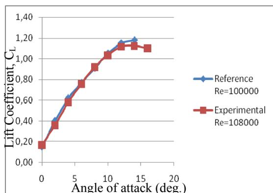
Fig. 6. Lift coefficient graph of the NACA 2415 airfoil
