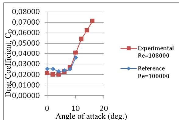
Fig. 7. Drag coefficient graph of the NACA 2415 airfoil
