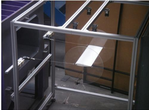
**Fig. 2. Location of scales in the aerodynamic balance**
