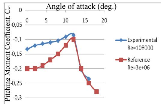
**Fig. 9. Pitching moment of the NACA 2415 airfoil**
