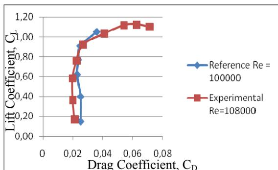
**Fig. 8. Drag polar of the NACA 2415 airfoil**
