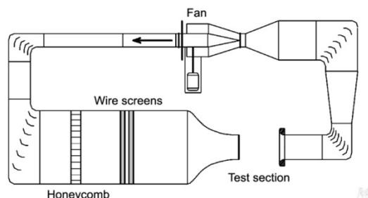
Fig. 1. Low speed wind tunnel.
