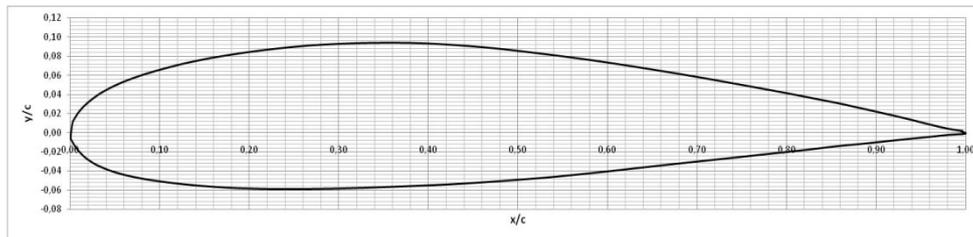
Fig. 4. NACA 2415 airfoil
