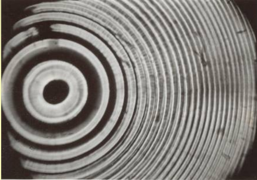
Microphoto of cross section of produced preform
